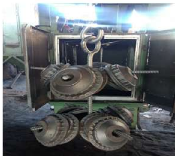
Fig 1. Existing Hanger with castings use in short blasting machine.
